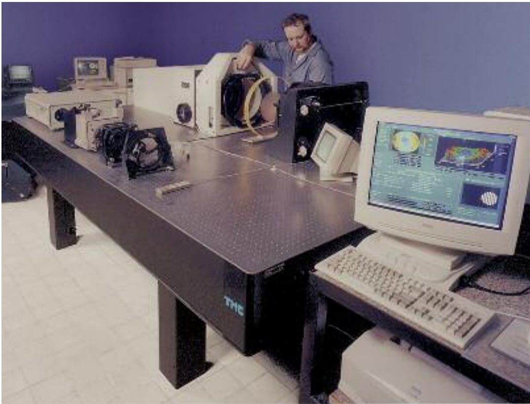
CleanTop® Optical Table supporting a Zygo Interferometer used for testing flatness of large optics. Photo courtesy of Quality Laser Optics
