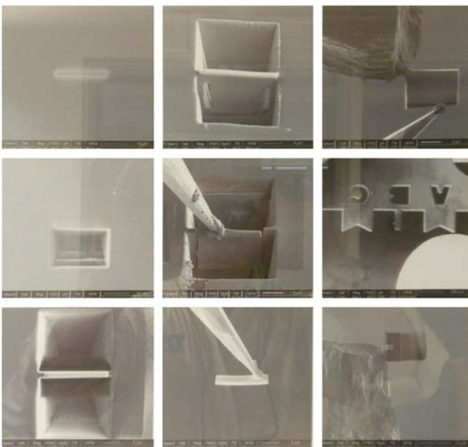
*SEM images of Step-by-Step Lift-out process (courtesy of PSU-CEMN)*
