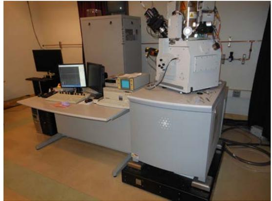
*FEI Strata™ FIB-SEM installed on TMC SEM-Base™*
