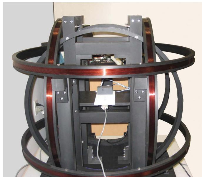
Figure 3. True Helmholtz Coils required for precision field creation.
