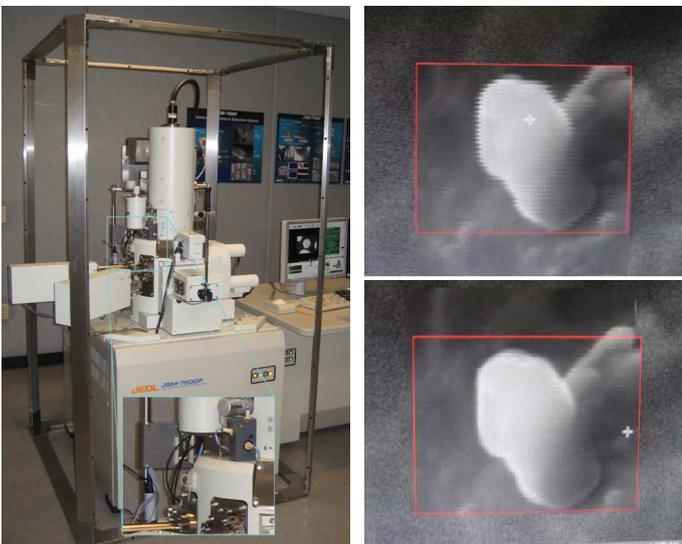
**Figure 1.** The left hand image shows a typical Mag-NetX installation with Mag-03IE70v1 sensor. In the top right image the B field is not suppressed. In the bottom right it is suppressed with the Mag-NetX system. Scanning Electron Microscope, Magnification 70k.
